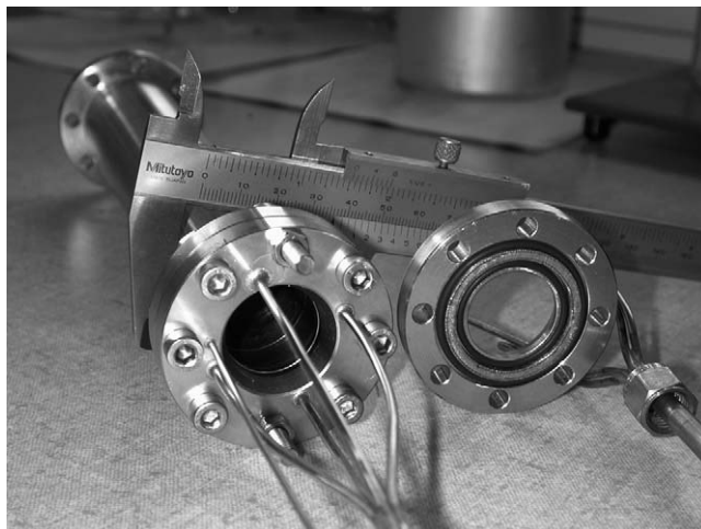
Fig. 3. Top view of annular type PROX reactor.
