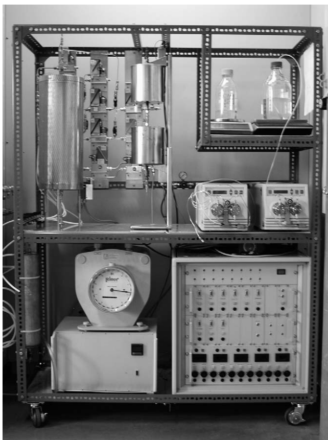
Fig. 4. Lab-scale gasoline fuel processor consisting of an autothermal reformer and a preferential oxidation reactor.
